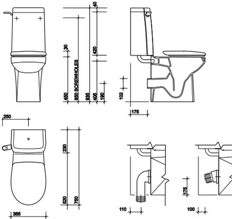
All measurements shown are in millimetres.
