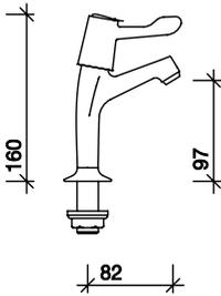
All measurements shown are in millimetres.
