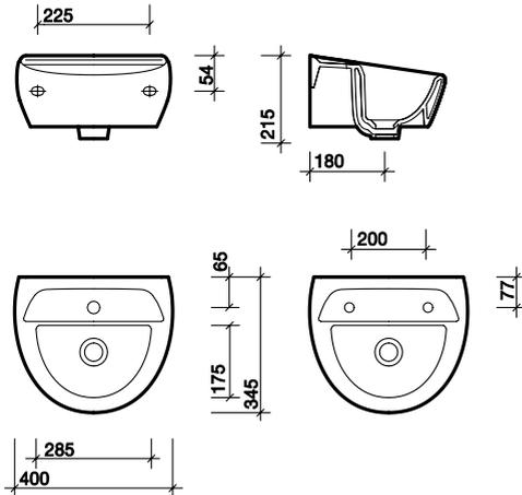
All measurements shown are in millimetres.
