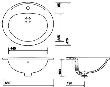
All measurements shown are in millimetres.
