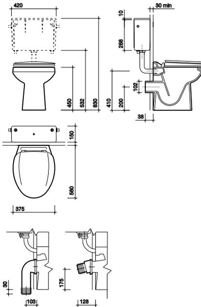
All measurements shown are in millimetres.
