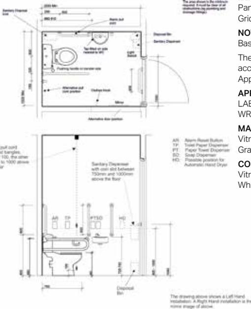
All measurements shown are in millimetres.
