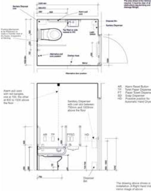
All measurements shown are in millimetres.
