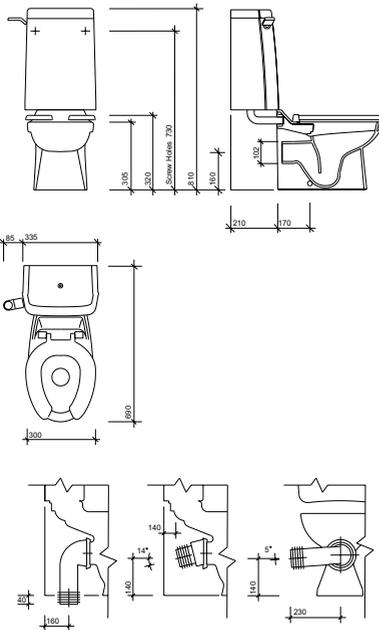
All measurements shown are in millimetres.
