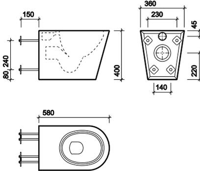
All measurements shown are in millimetres.
