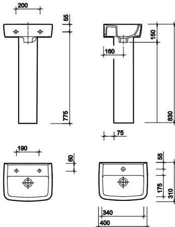
All measurements shown are in millimetres.
