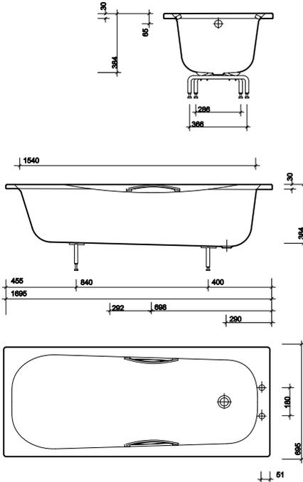
All measurements shown are in millimetres.
