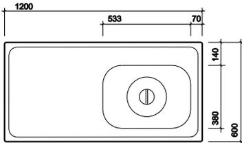
All measurements shown are in millimetres.
