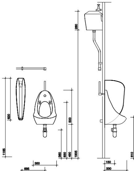
All measurements shown are in millimetres.
