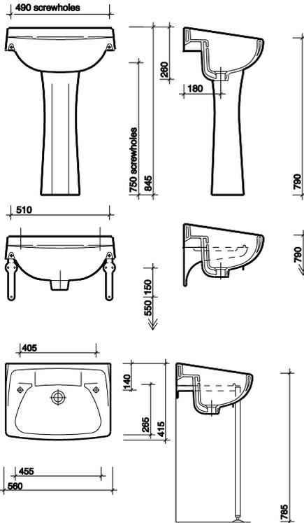
All measurements shown are in millimetres.
