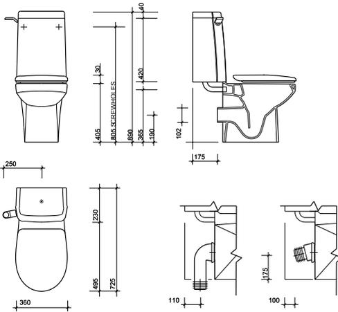
All measurements shown are in millimetres.
