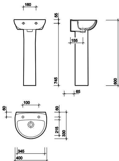
All measurements shown are in millimetres.
