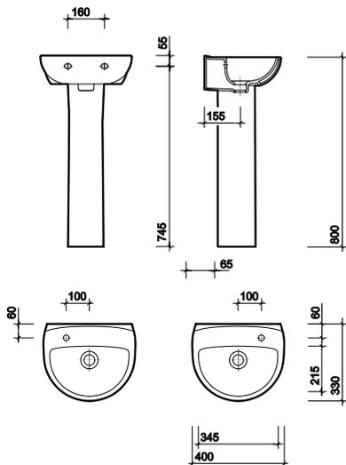
All measurements shown are in millimetres.
