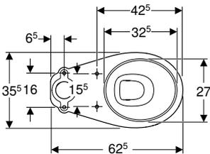
All measurements shown are in millimetres.
