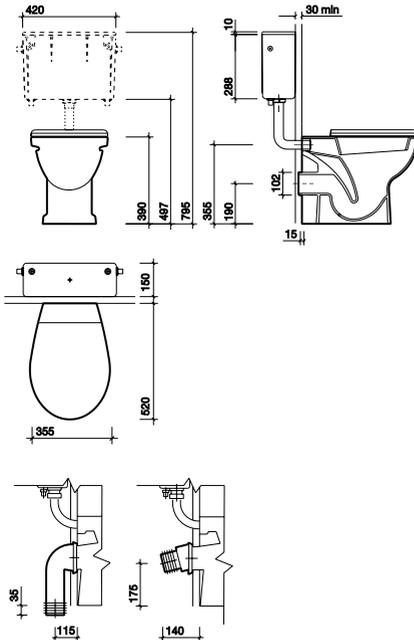
All measurements shown are in millimetres.
