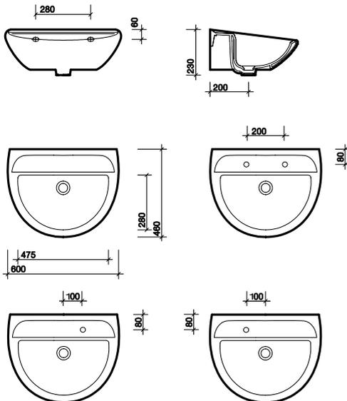
All measurements shown are in millimetres.
