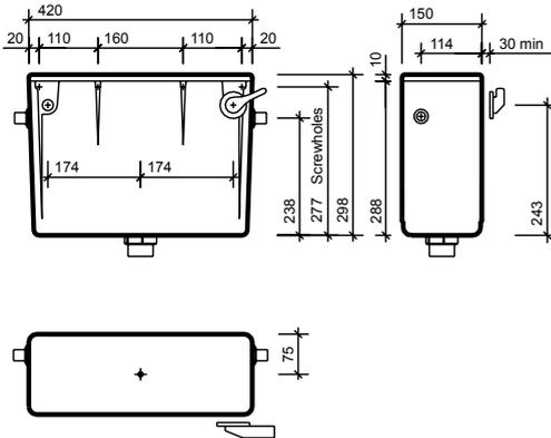
All measurements shown are in millimetres.
