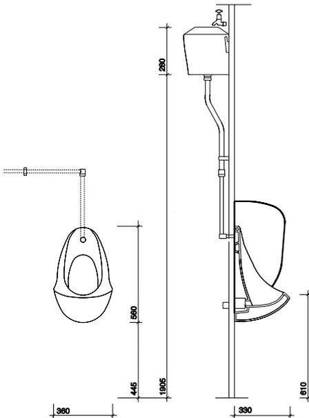
All measurements shown are in millimetres.
