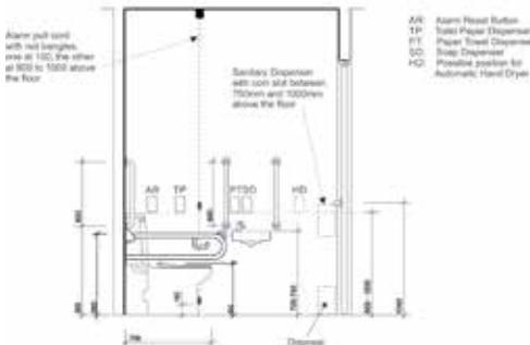
All measurements shown are in millimetres.
