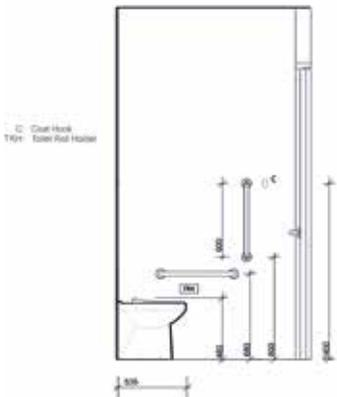
All measurements shown are in millimetres.
