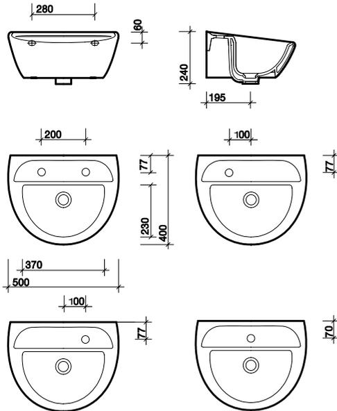
All measurements shown are in millimetres.
