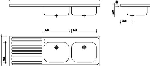
All measurements shown are in millimetres.
