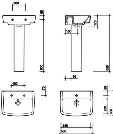
All measurements shown are in millimetres.
