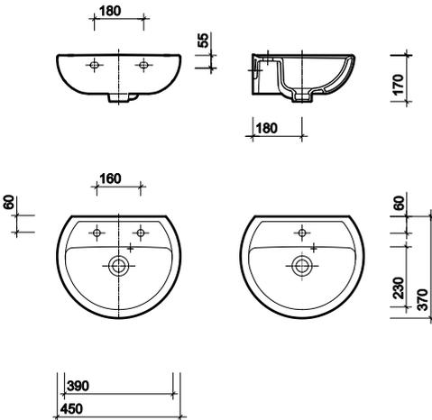
All measurements shown are in millimetres.
