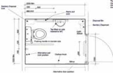
The drawing shows a Right Hand installation. It should be clear of all possible protrusions and storage fittings.
