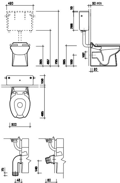
All measurements shown are in millimetres.
