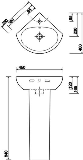
All measurements shown are in millimetres.
