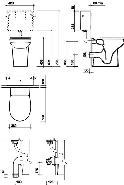
All measurements shown are in millimetres.
