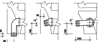
All measurements shown are in millimetres.
