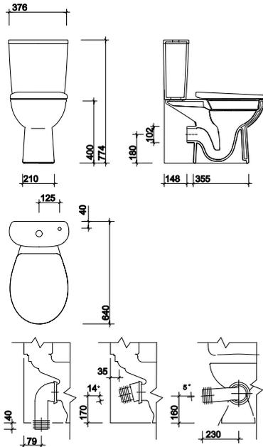
All measurements shown are in millimetres.
