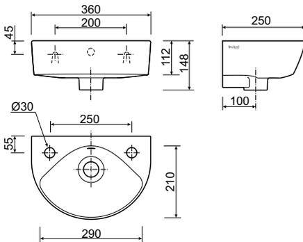
All measurements shown are in millimetres.
