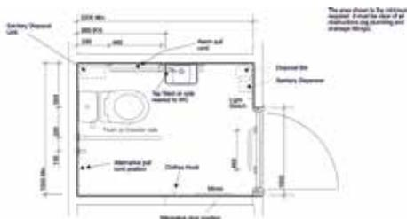
The area shown is the minimum required. It should be clear of all obstacles and protrusions.
