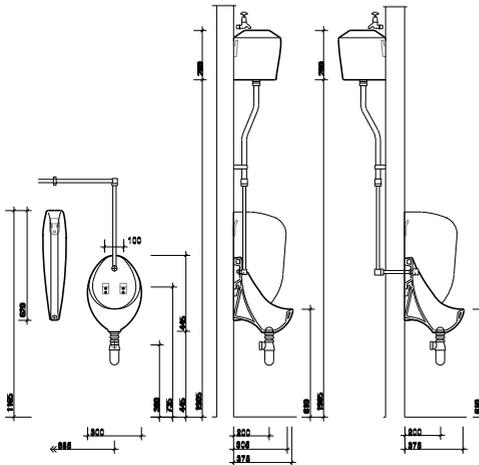
All measurements shown are in millimetres.
