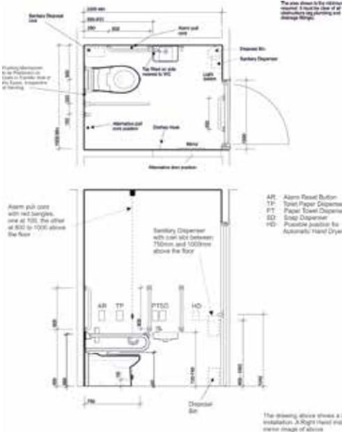
All measurements shown are in millimetres.
