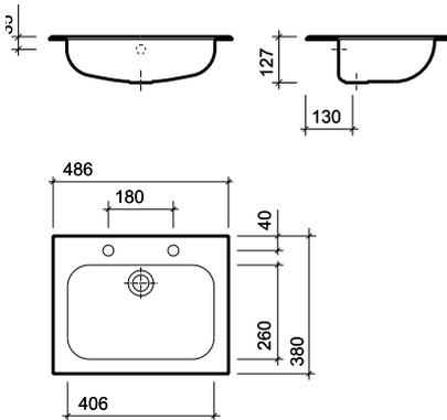
All measurements shown are in millimetres.
