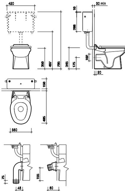
All measurements shown are in millimetres.
